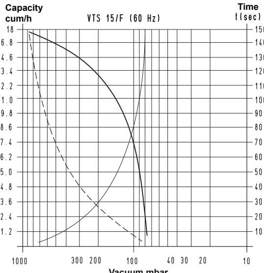
To calculate the emptying time of a volume  $V_1$ , apply the formula  $t_1 = \frac{t \times V_1}{100}$
